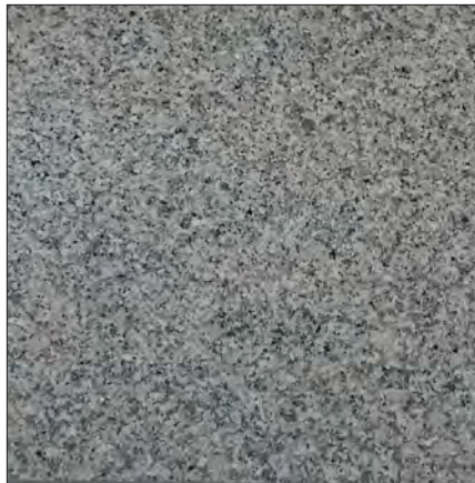
Granite - A hard rock, consisting of small, yet visible, grains of minerals, which can be highly polished or textured; used for walls, piers and street curbs; commonly in gray, black and pink.
