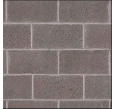
Concrete Block - A structural building material made by mixing water, cement, sand and aggregate, placing the mix in forms and hardening; commonly used for foundations, walls and piers.
