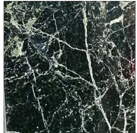
Marble - Typically fine grained and able to be highly polished; has a wide range of colors and patterns; used for steps and stoops, statuary and fine masonry.
