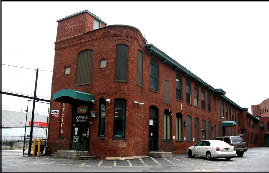
**BABOUR 9:** oblique view looking SE of 1890 addition along Prince St. Note the rounded brick detailing in the cornice and lintels.
